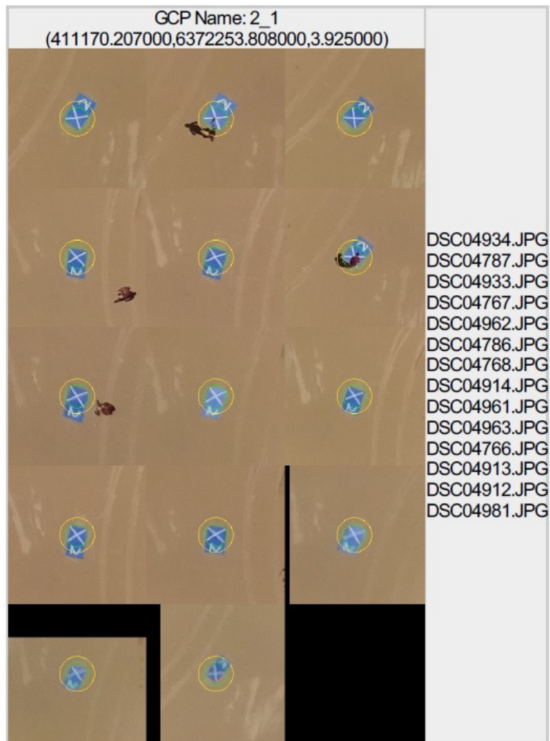
Figure 6 Example of procedure of Aero Trinagulation performed by the operator within PostFLight Terra 3d. The same target on the ground is seen by different orientation and angles and the operator has to adjust the suggested points (by the software, using coarse on-board GPS coordinates) and place them in the centre of the X displayed by the targets. This will allows PostFlight Terra 3d to model the camera distortion parameters and perform SfM-MVS routine to extract DSM and orthophoto.
